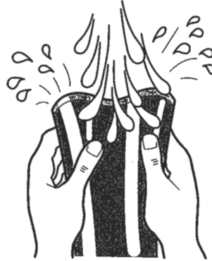
Figure 18: Typical air intake filter, also known as the coarse filter
